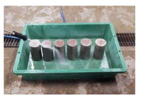
Research results of Professor Takafumi Noguchi have provided one solution for this issue. Spraying carbonated bubble water onto hardened cement revealed that the cement hardened because CO2 reacted with the calcium hydroxide in cement. Koizumi Seima Co., Ltd. became interested in the research results, and in 2021, concluded an exclusive license agreement for the patent held by the UTokyo. Koizumi Seima is planning to launch a device that sprays carbonated bubble water on cement.
